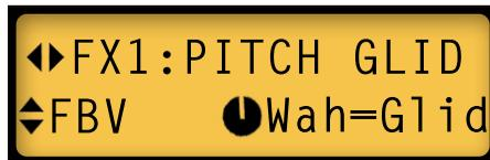
When Wah=Glid, if you switch the wah pedal off, the pedal will control volume as usual. If you switch the Stomp switch on, the volume pedal will switch to Pitch Glide again. Make sure your pedal volume is up all the way when you use the Stomp switch, however, because once the Pitch Glide takes over the wah pedal, you can't adjust volume unless you're using an external expression pedal for volume.
