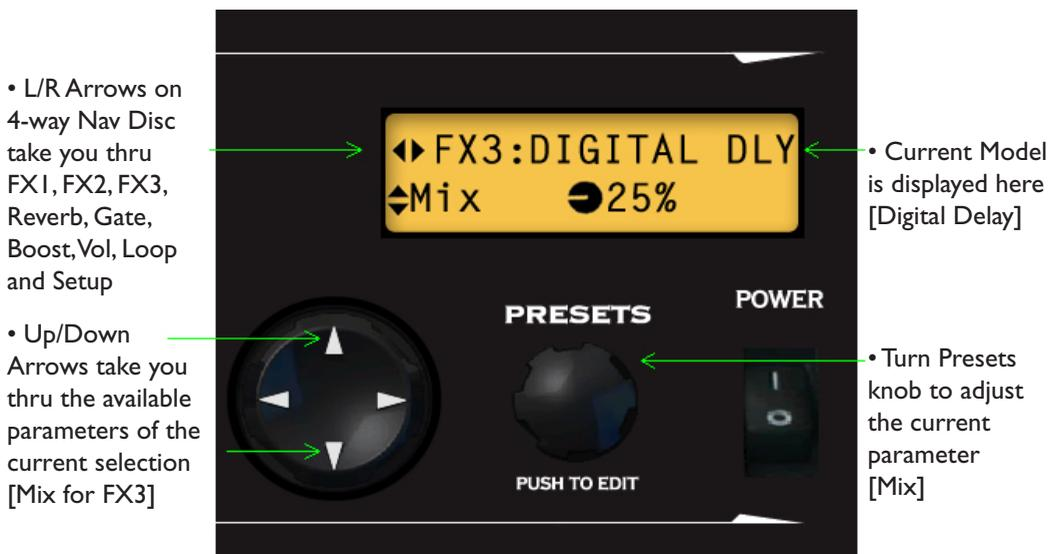
Use the L/R arrows to navigate thru the FX blocks. Use the up/down arrows to select the various parameters in each block. To adjust a parameter value, turn the Presets knob.
