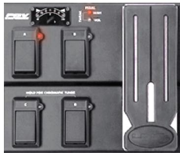
The FBV Express and FBV Express MK II will also control many Spider IV functions, including Tuner, Preset Select, Tap Tempo, and a few FX assignments for the pedal.
