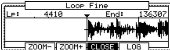
The waveform of the end point is displayed in the left of the waveform display, and the waveform of the loop point in the right, so you can adjust the loop and end points while checking the relationship of the waveform.
