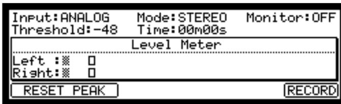
**03. Select the Input field, and select the recording source.**
