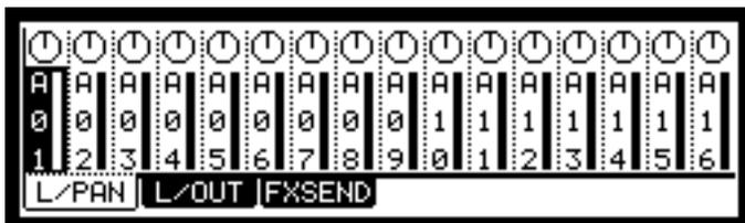
In this picture, each column indicates pad 1 through 16 from the left, and the currently selected pad is highlighted. The bar display on the bottom indicates the current level. Longer bars indicate a higher level.
