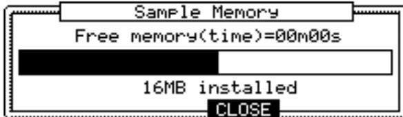
The Free memory field displays the time you can record with the current memory. Below it, the status of the memory is indicated as bar graph.
