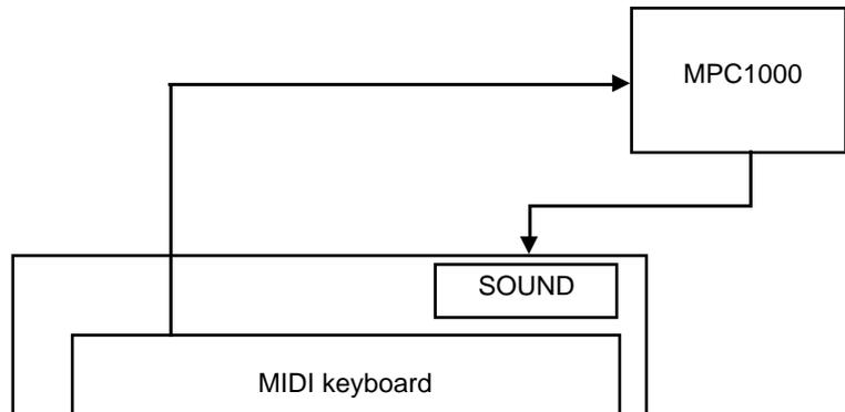
If your MIDI keyboard does not have a local control setting, deactivate the MPC1000's soft thru function. In this case, the MPC1000 will output only the data that is recorded on the track, not the incoming MIDI signal. However, if you do this, you cannot use some MPC1000 features, such as note repeat.
