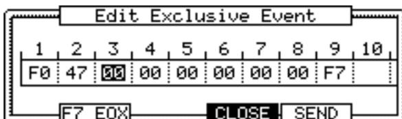
The data of each byte will be displayed. You can scroll through the display with right/left cursor keys.
