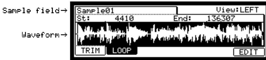
It displays the waveform of the whole sample, with the parts set by start/end points highlighted. If you select a stereo sample, you can select the channel (LEFT/RIGHT) to display in the View field.
