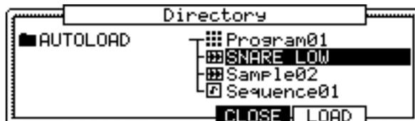
The folder selected in the folder field is displayed in the left of the directory list, and the files selected in the File field are displayed in the right of the list. In the picture above, the SNARE LOW file in the AUTOLOAD folder is selected. Each file has an icon according to their types.
